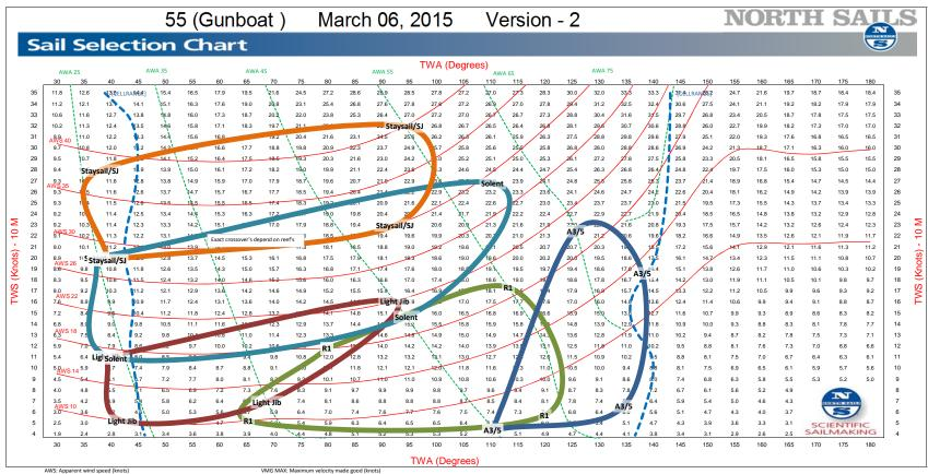
AWA: Apparent wind angle (degrees) TWS: True wind speed (knots)
