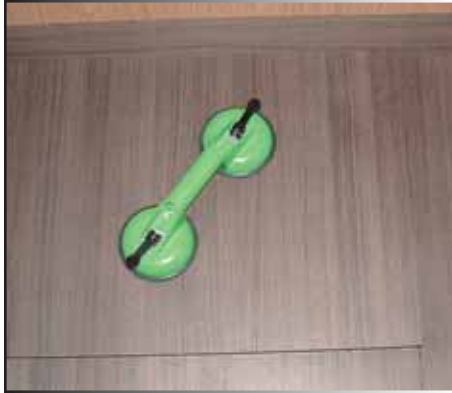
SUCTION PADS FOR THE FLOORBOARDS
