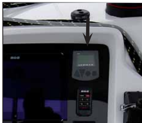
4 - ELECTRIC WINDLASS CONTROL + CHAIN COUNTER
