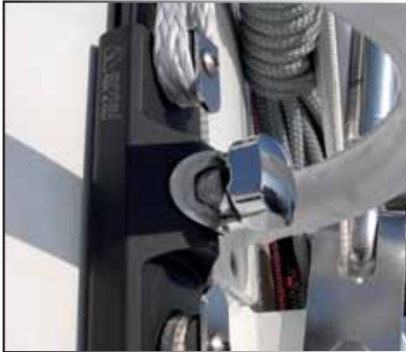
TRAVELLER BLOCKED IN OPEN POSITION
