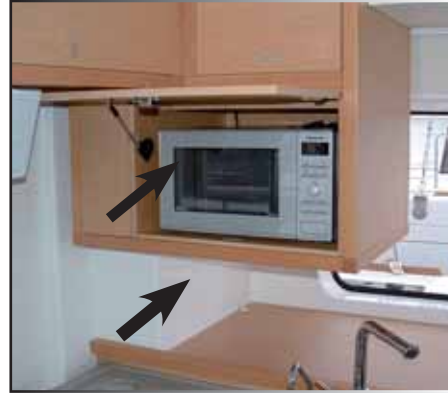
4 - LOCATION MICROWAVE OVEN + GAS SOLENOID VALVE SWITCH (US VERSION)
