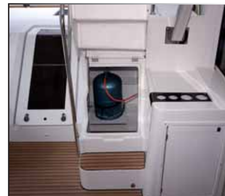
2 - LOCKER / STORAGE SPACE FOR GAS BOTTLES
