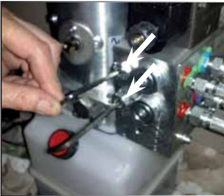
CONE-POINT SET SCREWS OF THE HYDRAULIC UNIT
