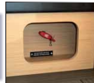
RELEASE PULL HANDLE OF 3 - PORT EXTINGUISHER 4 - STB EXTINGUISHER
