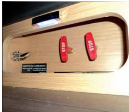
SHUT-OFF HANDLES FOR FUEL VALVES TO PORT
