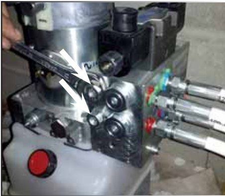
LOCKING NUTS OF THE HYDRAULIC UNIT
