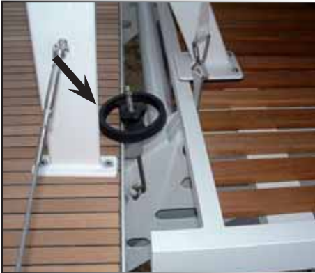
LOCK TURNBUCKLE OF TENDERLIFT
