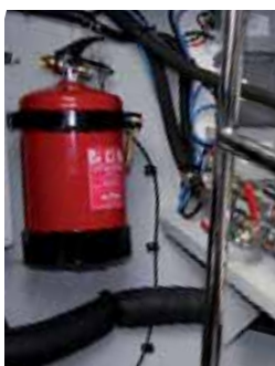
Fixed extinguisher system in the engine hold (access through the engine holds)
